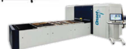
Vutek HS100 Pro Handles flexible or rigid substrates up to 3,2m and up to 5,08cm thick Expanded gamut CMYK pigments for world class Pantone matching Standard six colors (CMYK, lc, lm) plus two white channels 3,2 meter hybrid digital UV press handles up to 100 boards per hour, up to 70 boards per hour in Point-Of-Purchase mode (600dpi binary print mode)
